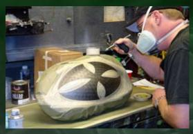
4. With the Machine turning finished, I spray the MC01 Aluminum Effect Kosmic Krome® over the Maltese Cross with my Iwata® TH-3 Fan pattern airbrush. Three (3) light coats are used to get the full aluminum effect.
