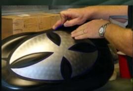
8. With the low edges, the graphics can now be properly pinstriped with little, if any fear of peaking, or separating when cleared later. The Maltese Cross is striped using the House of Kolor® U15 Lavender striping paint, with just a bit of KU150 mixed with the reducer.
