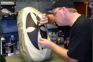
2. Using 3/4''  $3M^{TM}$  Crepe tape, I mask off the rest of the speed shape in preparation to painting.
